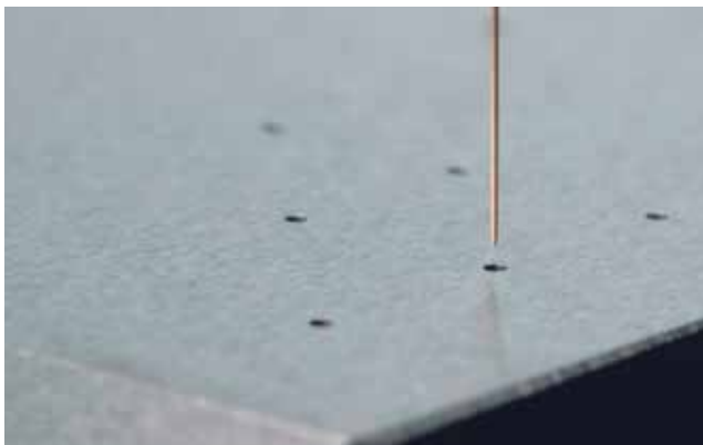
Left: Automatic wire threading of a 0.25 mm diameter wire into a 0.7 mm hole.
