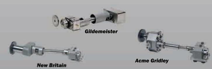
The thread milling operation is obtained by a particular cutting tool, which is helical shaped with the same pitch of the thread. This tool rotates at the same spindle's speed, the feeding stroke is radial, as the attachment is placed onto the lathe's cross slide. The thread milling unit can be used on aluminium, brass, lead free brass and steel (using solid carbide cutters or HSS); the thread can be located in the front side of the part and also behind a shoulder, near the collet.
