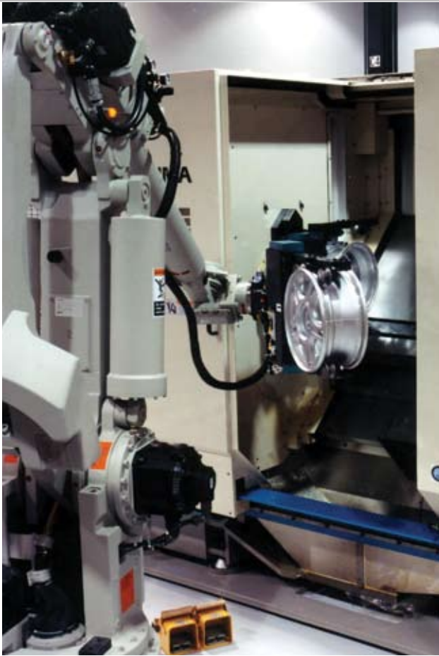
A Motoman SK120 robot unloads a machined wheel and loads a raw part into a CNC lathe. (Photo courtesy of Motoman, Inc.)
