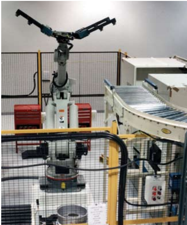
A Motoman SK120 robot with mechanical gripper loads/unloads wheels into/from two lathes in this machining cell. (Photo courtesy of Motoman, Inc.)
