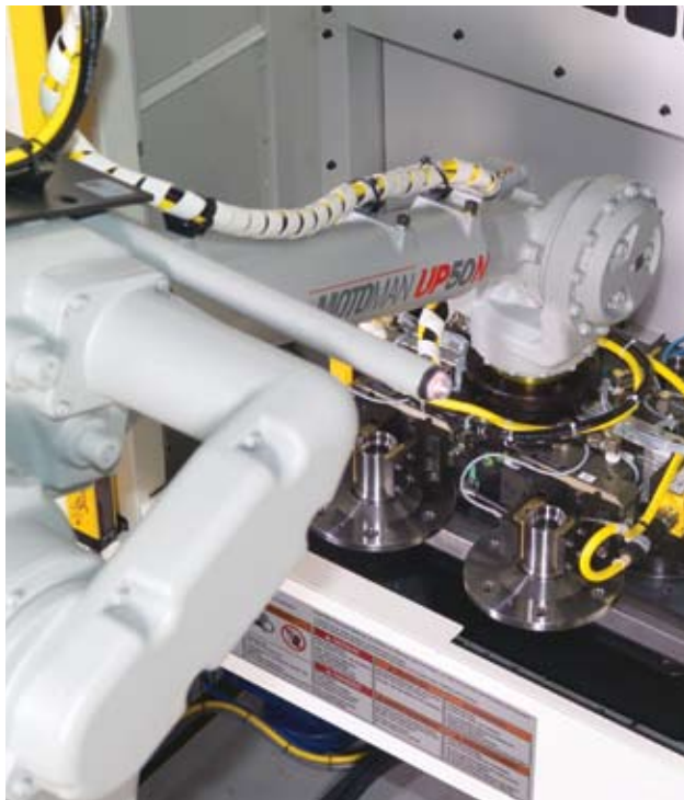
Closeup of Motoman UP50N robot loading a pair of wheel hubs in a machining center for a drilling operation. (Photo courtesy of Motoman, Inc.)
