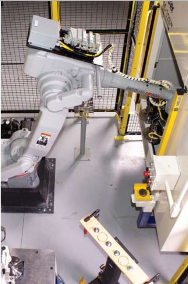
Motoman UP50N robot loads/unloads pairs of wheel hubs into/from two identical machining centers and a gauging fixture. (Photo courtesy of Motoman, Inc.)
