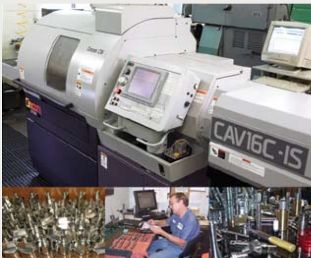
Citizen CAV16C Swiss turning center surrounded by representative parts and a Permac Inspector at work.
