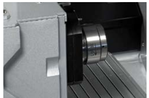
Close Up of the powerful 5 HP Sub-Spindle
