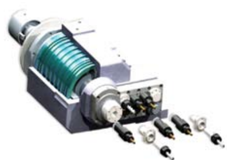
Oil cooled built in motors.
