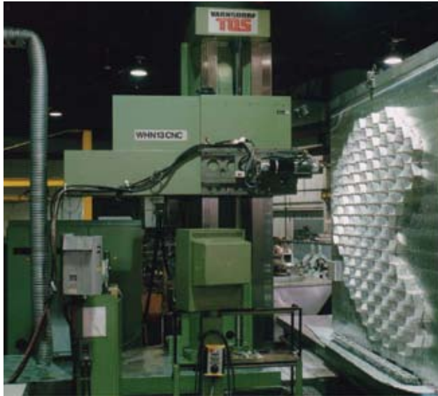
An auxiliary high speed spindle mounted on machining center finish-cuts a satellite honeycomb panel with 0.013 walls. This part starts out as a 4000-pound piece of aluminum, and weighs about 32 pounds when completed.
