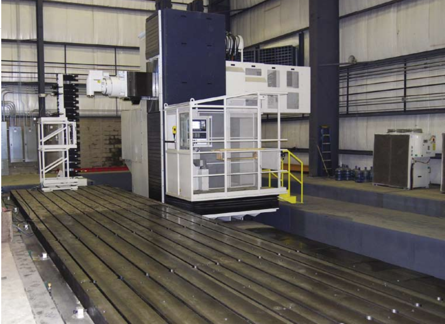
Above: Giddings FTR5000: The latest HBM from MAG is the floor-type FT and FTR Series for extremely large parts. The model pictured includes an optional right-angle head for additional machining flexibility.
