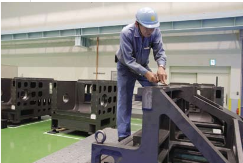
Mitsui Seiki factory worker preparing to hand scrape ways.
