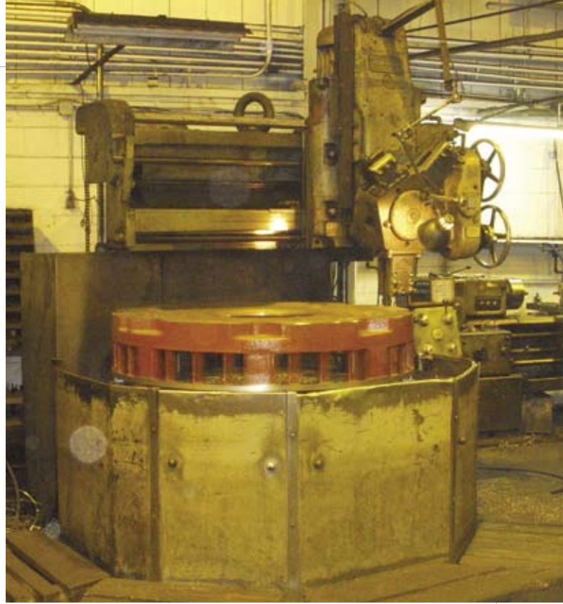
Above: This workpiece is a clutch for a press brake being machined on a manual, vertical boring mill.
