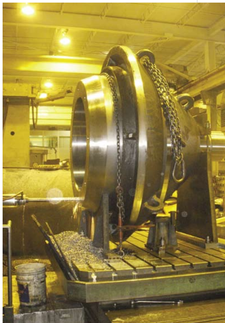
Above: This workpiece is for a stone crusher. It's being machined on a horizontal boring mill. Photo courtesy of Pride machine Co.
