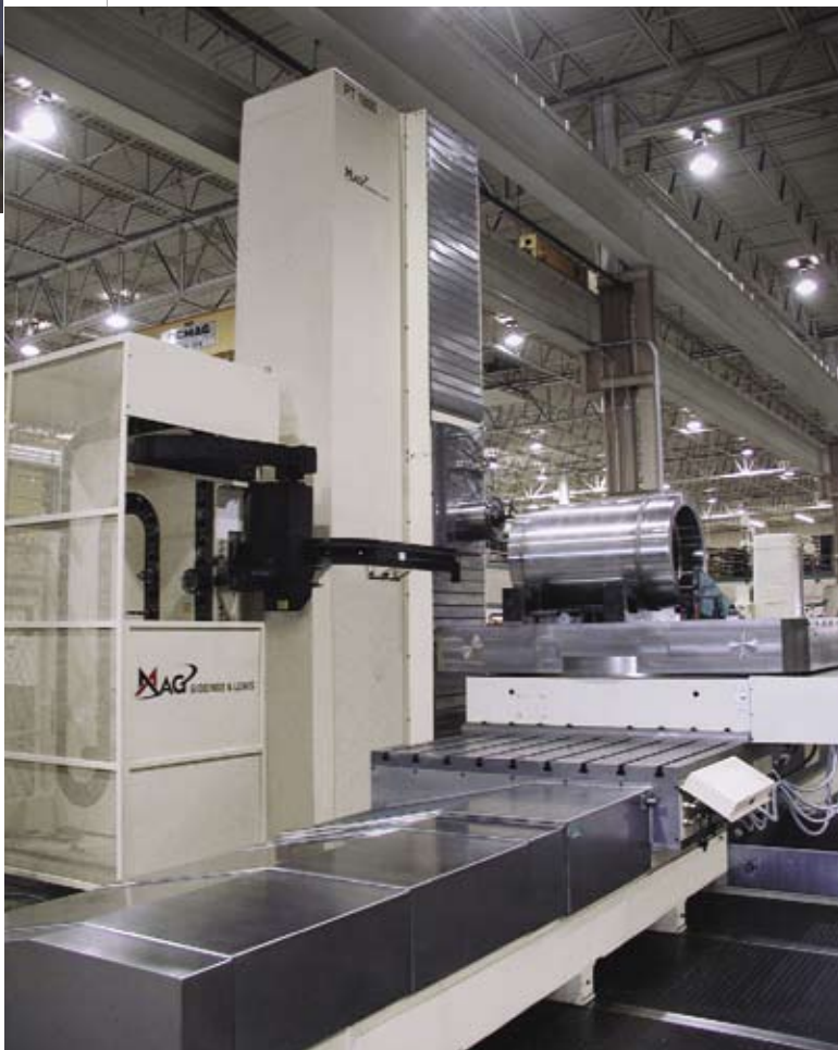
Above: A MAG PT Series plain table boring mill installed at Busch Precision in Milwaukee. Photo courtesy of MAG Giddings & Lewis.
