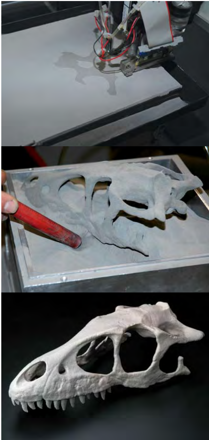
Above: Fabricate by 3D Printing: (1) Three-dimensional CAD information is converted into powder metal, ceramic or sand layer-by-layer by bonding loose particles with binder, (2) creating a physical object identical to the original CAD file, (3) that upon finishing results in a final Art, Part or Tool.
