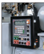
3. CS 2001 microprocessor control
