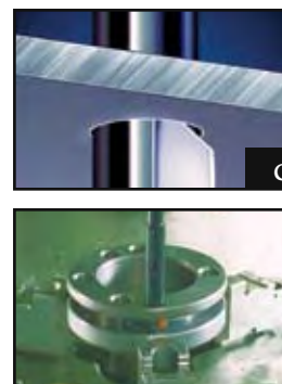
PHOTOS ABOVE: a,b,c. Hole deburring tool deburrs front and back of the hole. d. Micro deburring tool from E-Z Burr Photo courtesy of E-Z Burr Tool Company.
