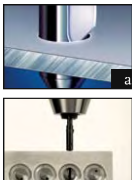
PHOTOS ABOVE: a,b,c. Hole deburring tool deburrs front and back of the hole. d. Micro deburring tool from E-Z Burr Photo courtesy of E-Z Burr Tool Company.
