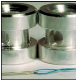
Small parts deburred with thermal energy method.
