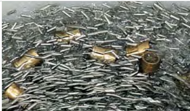
Magnetic deburring in action. Photo courtesy of Earth-Chain USA
