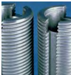
Parts before and after deburring by electrochemical machining.
