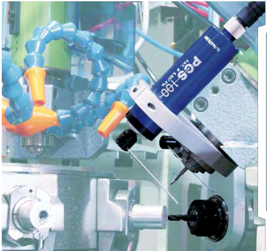
PCS Positive Contact Tool Monitor from TPS International, installed on a transfer machine. Photo courtesy of TPS International.
