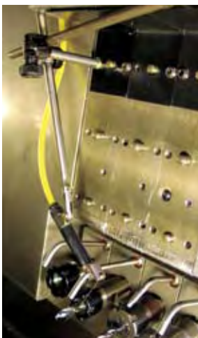
Installing the Detector Type 202 broken tool sensor from SPC Innovations. Illustration courtesy of SPC Innovations.
