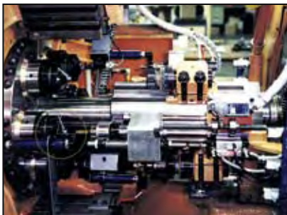
TPS International PCS tool monitoring system, showing sensor, control box, sensing cable and mounting bracket.
